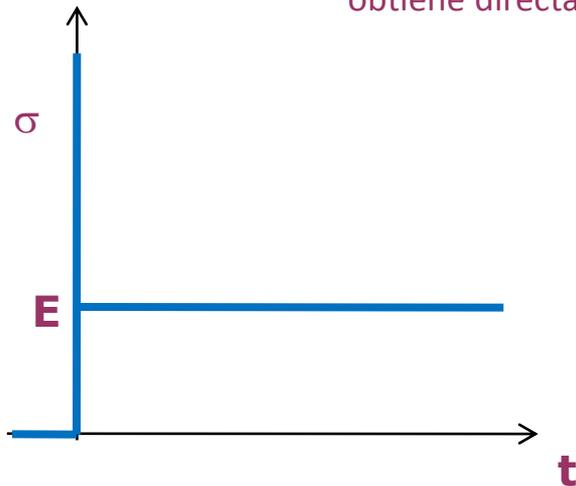
$$Y(t) = \sigma(t) = E + c\delta(t) \quad \forall t \geq 0$$
